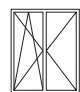
Ventana y balconera a la francesa oscilobatiente French + tilt and turn window and balcony door
